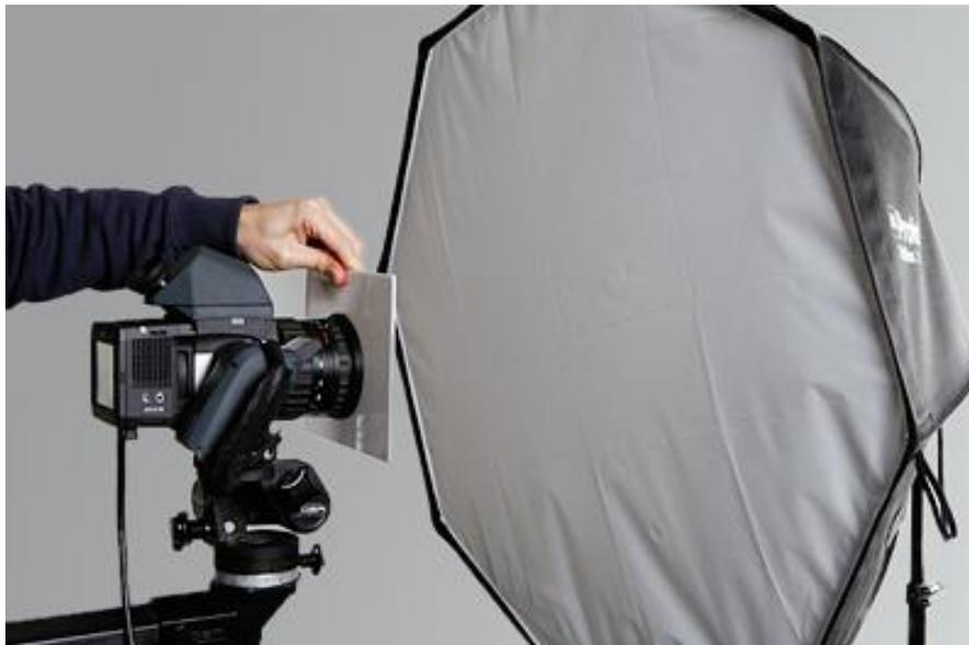
With this setup, you can now create the lens calibration file using Leaf Capture's calibration wizard.
