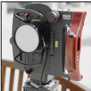
**Note:** To achieve good results, do not move the camera or lens position, or change the aperture before taking the diffuse calibration shot.
